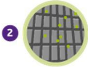
Formations of lead sulphate crystallise and become inert.
