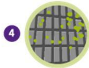
The sulphate then forms active sulphuric acid, and lead is free to run again.
