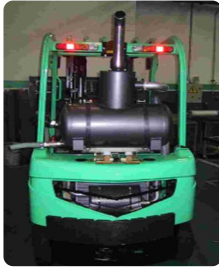
EXHAUST PARTICLES CLEANING SYSTEM
