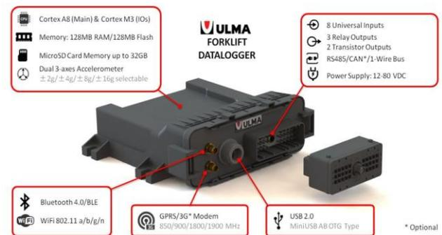
Fig. 5. Embedded data logger developed for transportation after an analysis of the existing HW solutions.
