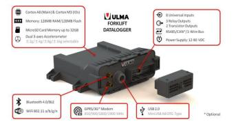
Fig. 5. Embedded data logger developed for transportation after an analysis of the existing HW solutions.
