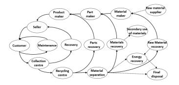
Fig. 7. Graphical simplification of Ricoh Comet circle <sup>TM4.</sup> The graph shows the increased steps (and often cost) associated to a scenario of zero-waste and re-manufacturing concepts. The more to the right in the activity cycles, the higher cost these activities represent with respect to operation. In order to enhance customer satisfaction it is necessary to extend at maximum the left inner circle
